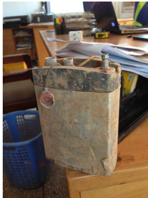
Figure 2–4: Flow and Pressure Data Logger
